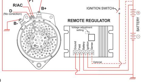
\*All 200 Series with internal V. Regulator are self-excited. If the vehicle has an ignition (excite) circuit, cap the excite wire as it is not required.
